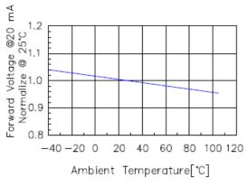
Fig 3. Forward Voltage vs. Temperature
