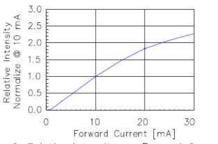
Fig 2. Relative Intensity vs. Forward Current
