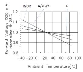
Fig 3. Forward Voltage vs. Temperature
