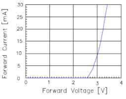
Fig 1. Forward Current vs. Forward Voltage
