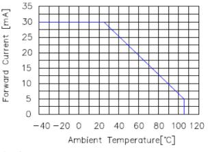
Fig 6. Forward current vs. Temperature
