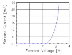
Fig 1. Forward Current vs. Forward Voltage
