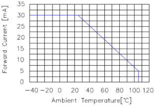
Fig 6. Forward current vs. Temperature
