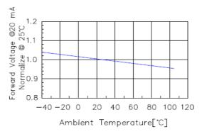
Fig 3. Forward Voltage vs. Temperature
