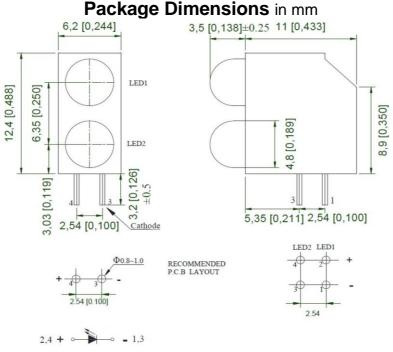
Figure 1. INH-48DXX60 series Package Dimensions
