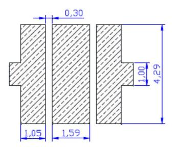
Figure 1. IN-C45PPBTLU1 Recommended Solder Pattern
