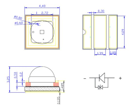
Figure 2. IN-C45PPBTLU1 Package Dimension
